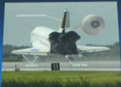
Endeavour comes in for a landing, with the speed brake open to slow down the orbiter.
