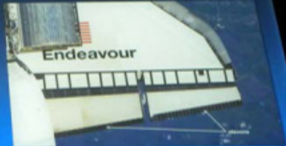
This close-up of Endeavour 's wing, taken from the International Space Station, shows the elevons in detail. Elevons are a unique feature: they partly resemble flaps on planes. The elevons and the elevons therefore can flap that move a plane up and down, and elevons flap control a plane's rolling motion. Elevons do both of these jobs.
